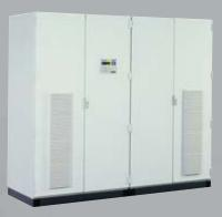
The AT 1600 is a high current, four-pole, three phase transfer switch. The use of oversized thyristors allows a fuseless design. The AT 1600 is available in a cabinet complete with isolation and bypass switches. An electromagnetic interlock of the bypass switches ensures a safe operation.
